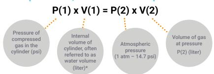
For example, a 300-size cylinder is filled at 2600 psi. What is the gas volume from the cylinder?
