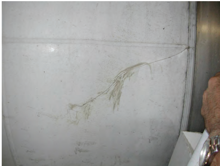
Figure 8.1 Cracking on the mixing drum of a ready-mix truck
