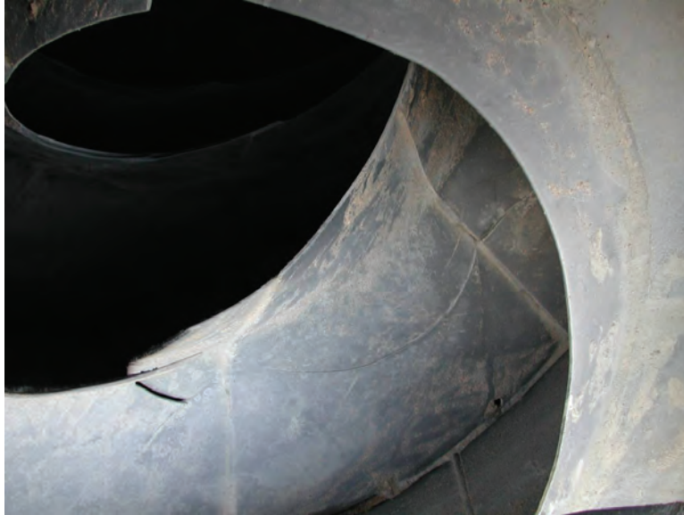
Figure 8.2 Cracking caused by liquid nitrogen dosing on a mixing drum fin
