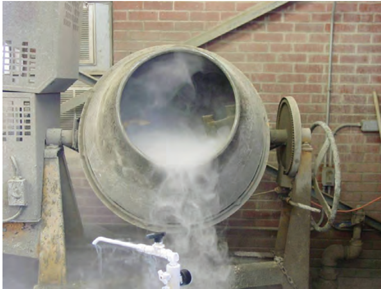
Figure 3.3 Vapor flows freely from the uncovered mixer
