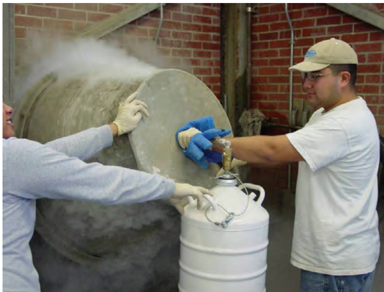
Figure 3.4 Plastic cover with hole in the middle for liquid nitrogen dosing
