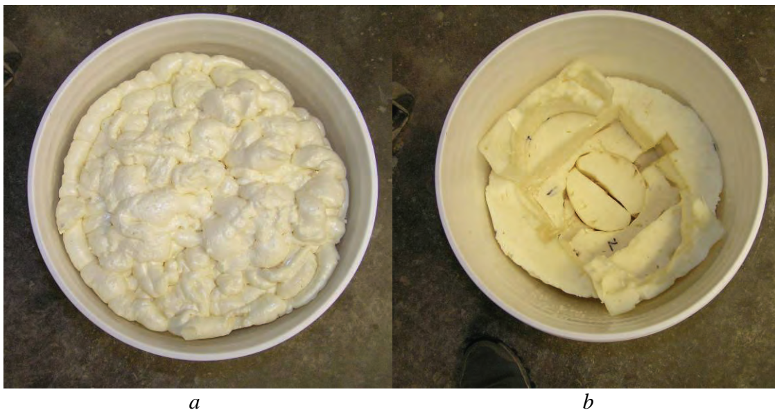
Figure 6.1 Insulating chambers made for set time specimens
